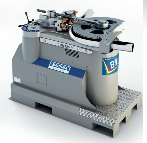
Tube and Pipe Bending machine BM125, non mandrel, electric, semi-automatic
